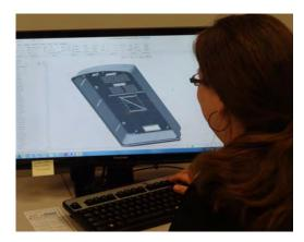
analysis and experiential knowledge, our engineers will evaluate how the resin will flow into the proposed tool design, fill the cavity, pack, cool and eject. The DFM process ensures the product is can be created while still meeting the quality requirements as designed, thus avoiding costly downtime and tool revisions.
