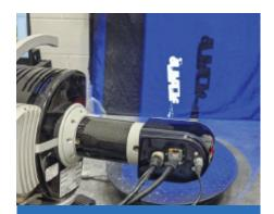
Ferriot's Aicon SmartScan uses blue-light technology to scan an injection molded part. Blue-light 3-D scanners offer better precision, accuracy and higher-quality outputs than white-light scanners, laser scanners and CMMs.
