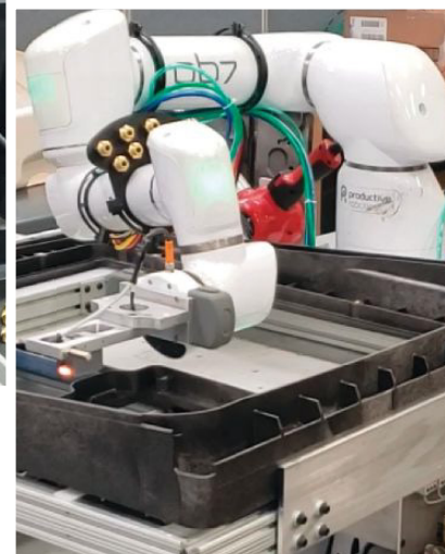
Left , at Ferriot Inc., a tray fabricated by the company's automation department holds a plastic part, and is guided under an ultrasonic welder by a cobot. Below , a cobot that is integrated with a vision system places an insert into a part.
