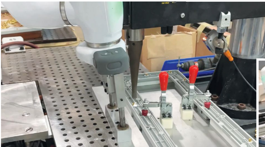
Left , at Ferriot Inc., a tray fabricated by the company's automation department holds a plastic part, and is guided under an ultrasonic welder by a cobot. Below , a cobot that is integrated with a vision system places an insert into a part.
